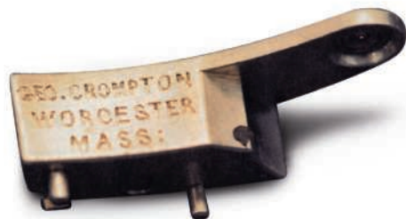
Third wheel bridge, hand-engraved: Geo. Crompton, Worcester, Mass
